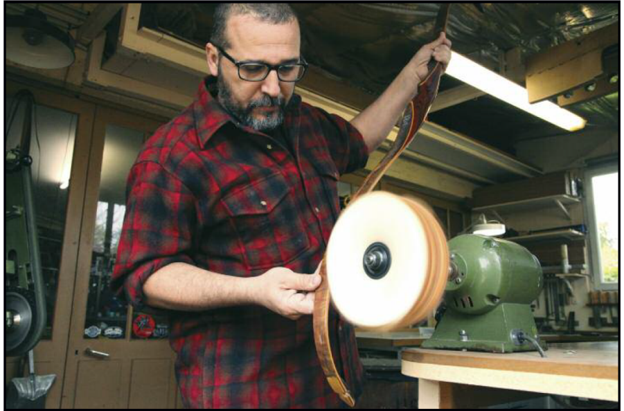
When the marine epoxy finish is dry, the bow is sanded with 1500-grit wet sandpaper and then polished.
