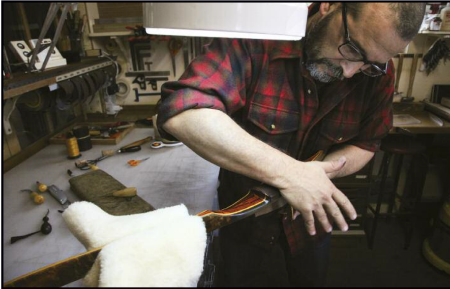
After a final inspection, the leather grip and rest are applied.
